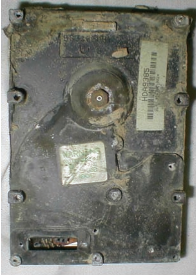
A data drive that fell from the space shuttle Columbia when it was destroyed in 2003 is shown. During Columbia’s fateful final mission, the drive had been used to capture data from a scientific experiment on the way xenon gas flows. Photo courtesy of Kroll Ontrack Inc.
